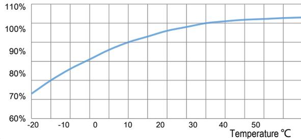
**Capacity Retention Characteristics**
