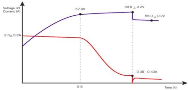
**Phase 1:** The Max. charge current is 2.0A, and the charge voltage is gradually risen up to 57.6V;
